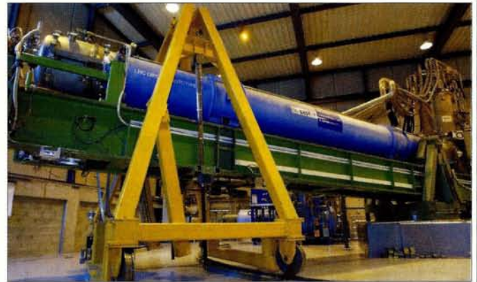
The CAST experiment at CERN, which is looking for axions from the Sun. It uses a prototype magnet for the Large Hadron Collider combined with particle-physics detectors and X-ray techniques from space-born experiments.
