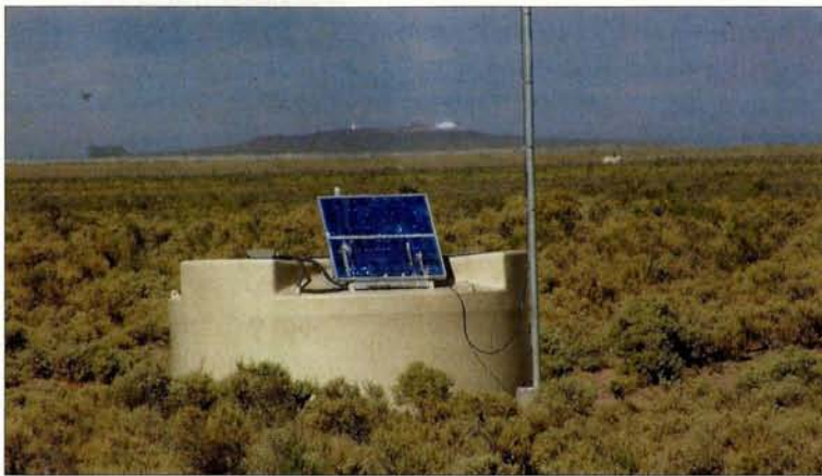
Combines techniques used in earlier experiments to study cosmic-ray air showers links such as the one on the right, detect Cherenkov radiation produced by high-energy particles. Nighttime optical detectors housed in larger buildings (left) record the faint light fluorescence of atmospheric nitrogen. (Photos: Pierre Auger Laboratory.)
