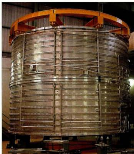
Two modules of the CMS solenoid at the manufacturers, Ansaldo, in Italy; the first module is the lower of the two. (Photo: INFN.)
