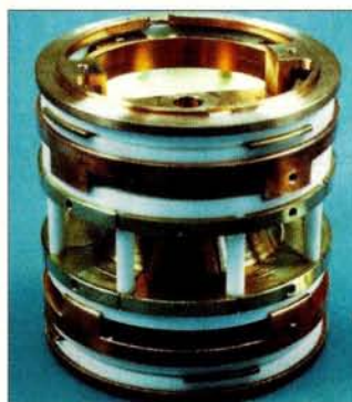
Far left: the vessel used for liquid nitrogen and helium cooling of the superconducting magnet coils and the detector system in ISOLTRAP's precision trap. Left: the precision trap (5 cm diameter), which sits inside the superconducting magnet.
